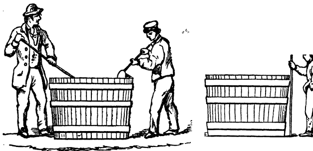
Fig. 177. Tossing and packing Tin Ores. (Henderson.)
